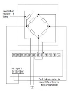
Contacts 2C and 2D on the PSU module can be manually shorted as in above drawing or they are automatically shorted by PnEL or PEL.I = Dn.
